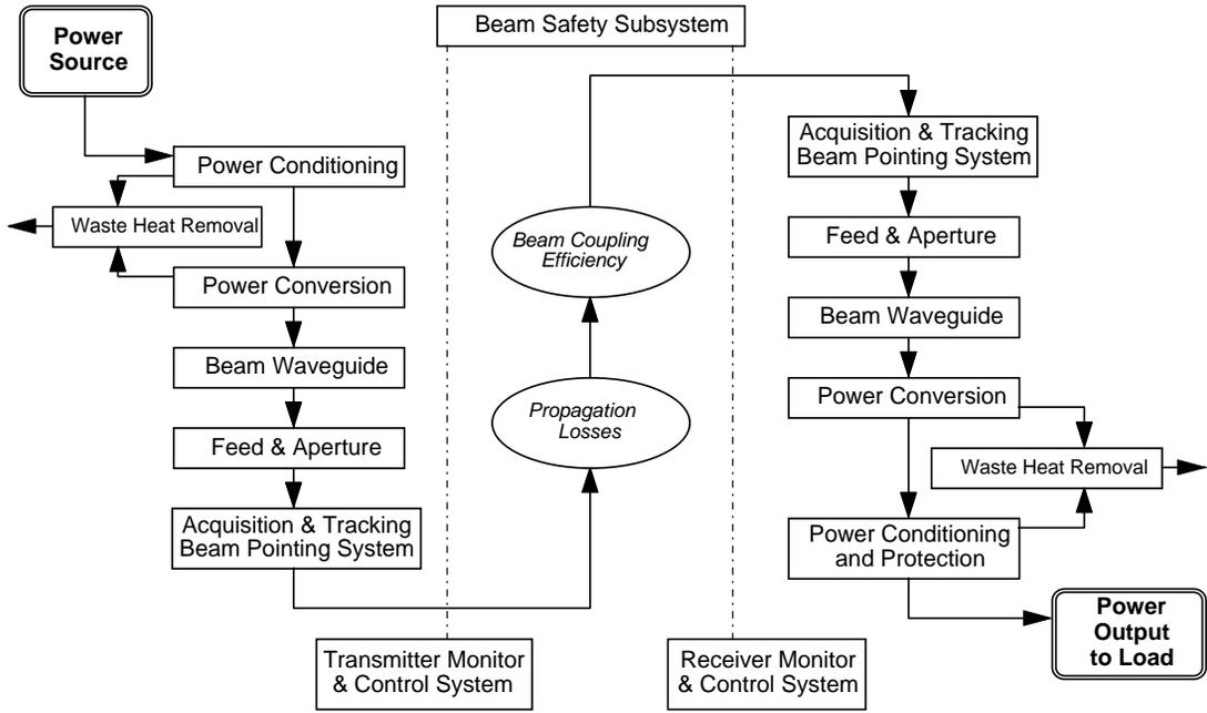
Fig. 1. Generic diagram of technical challenges associated with wireless power transmission.
