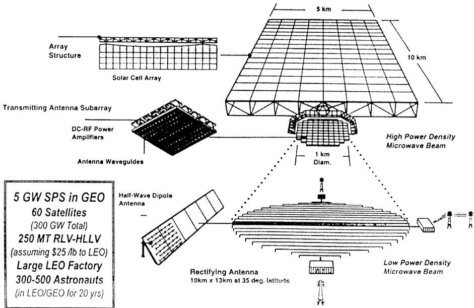
Fig. 2. 1979 SPS Reference System Concept: 5 GW power output, geostationary Earth orbit-based systems.
