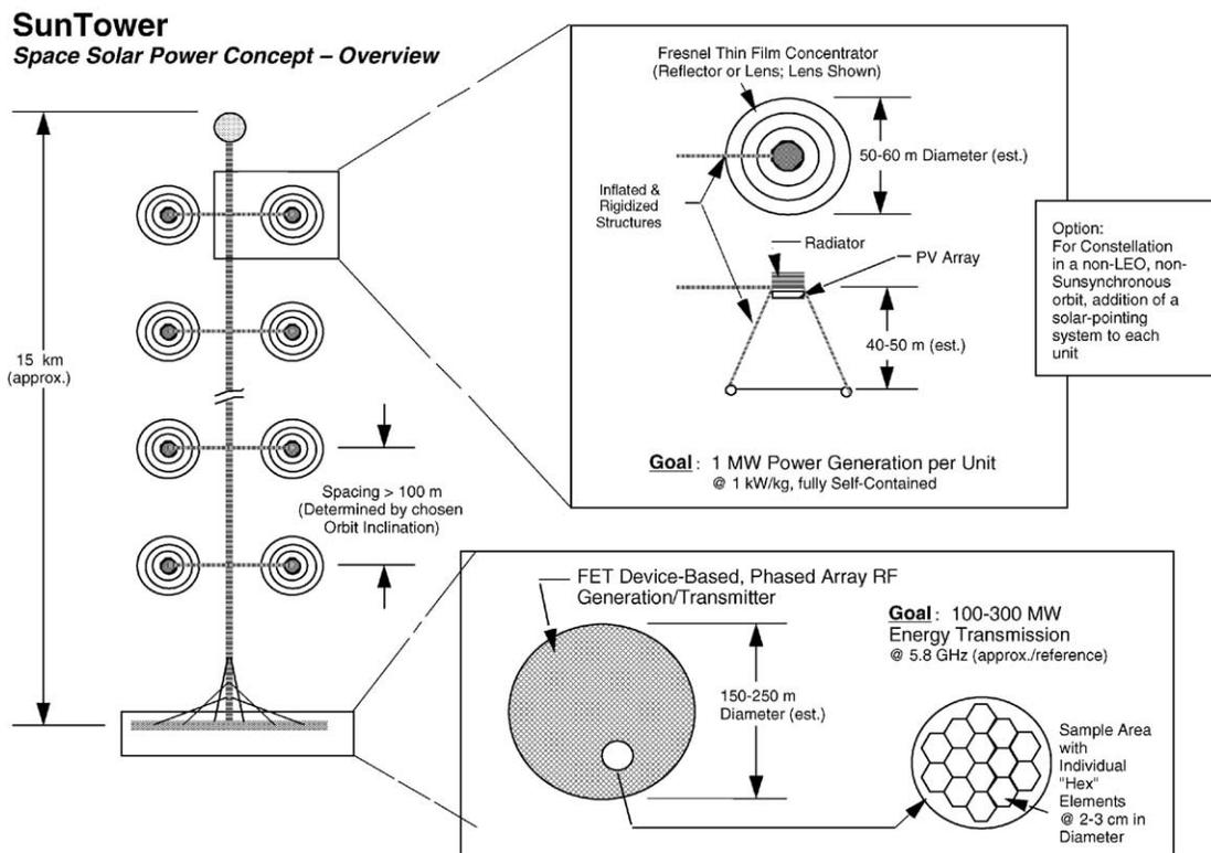
Fig. 3. The "SunTower" solar power satellite system concept.
