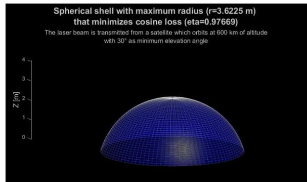
Fig. 11 Optimal receiver shape – 600 km case
