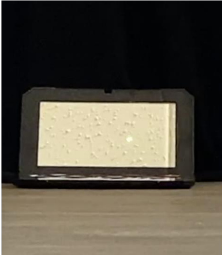
Fig. 5. High power 532 nm laser scattering off of a generic mirror
