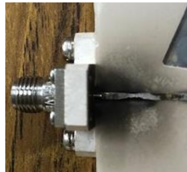
Fig. 8. The burnout of the connector
